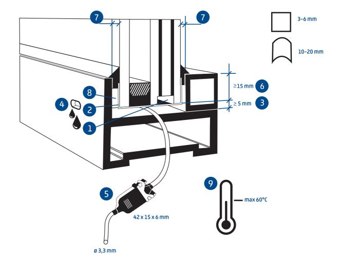
1 VISUAL CHECK: The glass pane is to be checked for any damage and malfunctions. SILATEC panes have a circumferential cladding tape which may not suffer damage. Faulty panes may not
